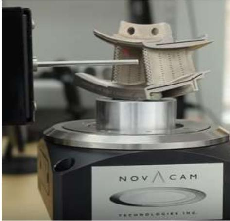
**Figure 8** A rotational scanner with a small-diameter optical probe inspects cooling holes on the inner surface of a stator blade.
