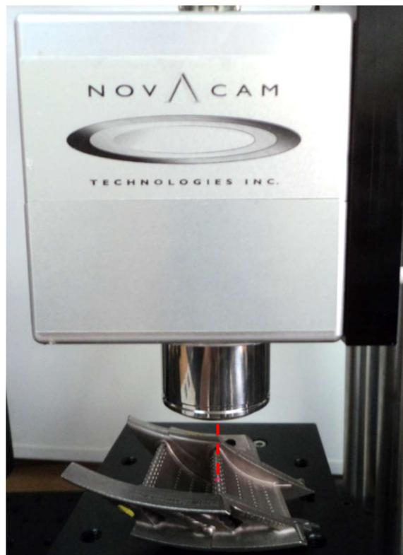
**Figure 7** The SurfaceInspect galvo scanner inspects cooling holes on the outer surfaces of a stator blade (nozzle guide vane).
