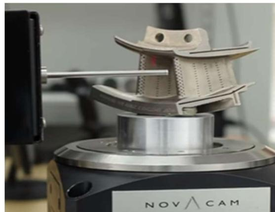
**Figure 7:** Novacam rotational scanner spins a small-diameter probe as it acquires the inside surface of a stator blade. The ID, including its cooling holes, is acquired as a dense spiral of 3D points.
