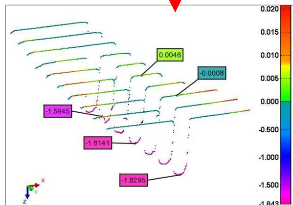
**Figure 2:** This detail indicates the data density of the 3D point cloud: a height profile containing 400 3D points was acquired every 1 mm along the length of the EDM slot. The height values are relative to the EDM slot upper edge and are noted in mm.
