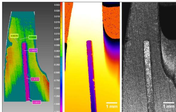
**Figure 3:** Alternate views of the EDM slot derived from higher-density scan data. From left to right: top view of the slot and the surrounding surface with colour mapping of the depth; height image; intensity image.
