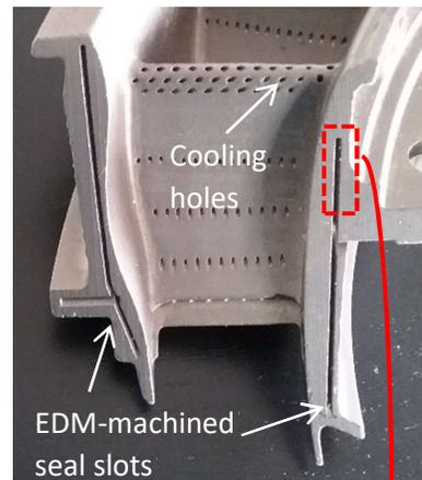
**Figure 1:** This stator blade features EDM-machined seal slots that are  $\sim 30$  mm (1.2") long, 0.4 mm (0.0157") wide and  $\sim 1.8$  mm (0.07") deep.
