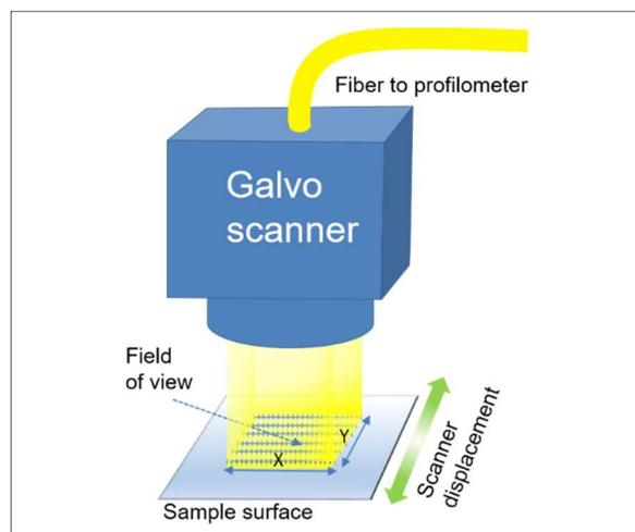
**Figure 4:** Novacam's optical galvo (raster) scanners come in several sizes of field-of-view.
