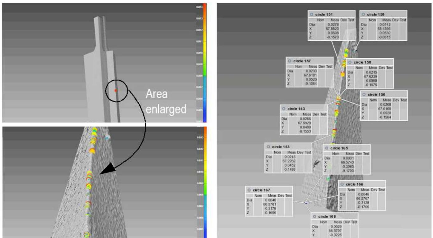
**Figure 3:** Users can zoom from an on-screen rendering of the drill bit (top left) into the edge area selected for analysis. The enlarged edge segment (bottom left) shows a colour-coded deviation map of the edge sharpness. On this micron-precision deviation map, the user may choose to view edge radii measurements at various points of analysis (right). The measurement units are user configurable.
