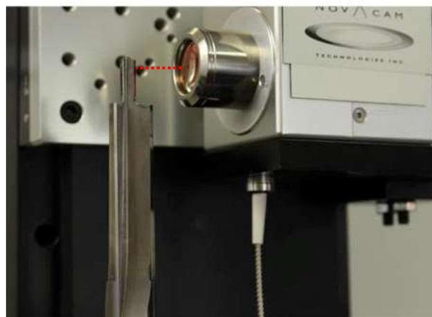
**Figure 2:** A machining drill bit (top left) is mounted on rotating chuck (top right). The tool is scanned by the galvo scanner, which in this configuration is mounted on a Z-stage (bottom left and right). The optical signals are processed by the profilometer.
