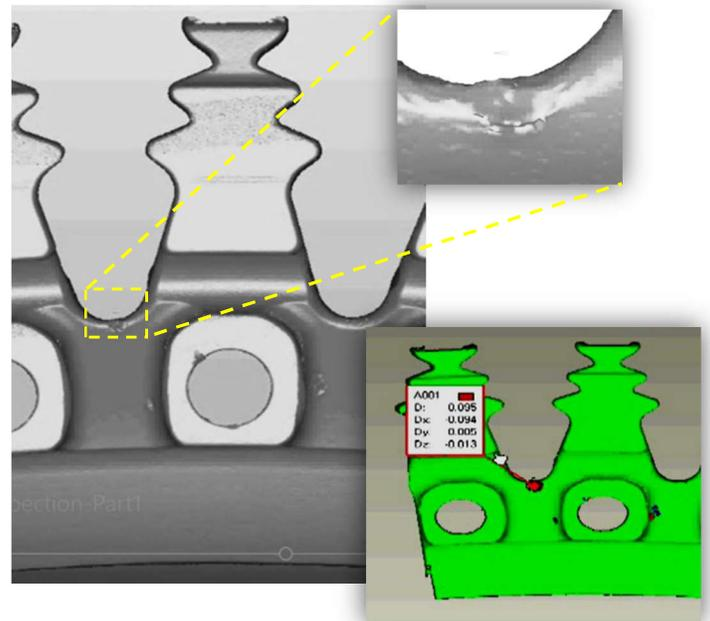
**Figure 1:** A chamfer defect is detected on the fir-tree base of a jet engine turbine
