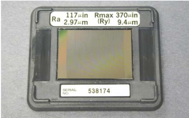
**Figure 3:** Mitutoyo roughness gage block
