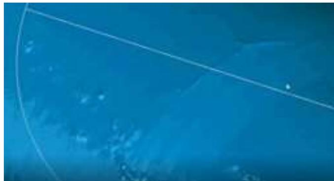
Figure 3: Users can zoom in further to examine barrel ID surface details.
