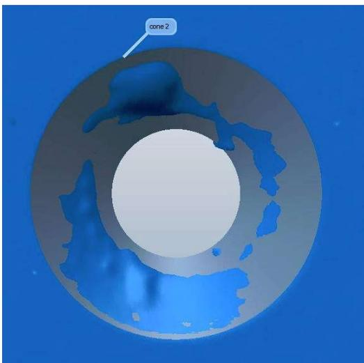
**Figure 7:** Variability of the 3D actual countersink (blue) from the spec (gray)
